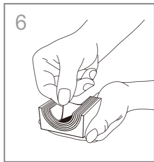
Step 6: Peel off the reducer of the module according to the outer diameter of the cable/pipe to adapt the inner diameter to the outer diameter of the cable/pipe.
